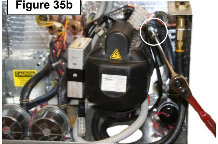
1. The Diesel-Burner is secured to the Hydro-Hot with two nuts that can be loosened, and swung out of the way by using a 10mm socket wrench with a 10 inch long extension.
