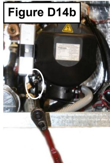
**NOTE: When reinstalling the diesel burner be careful not to damage the photo disc or bend the electrodes. Also, be careful to not pinch any wires between the burner and the Hydro-Hot Tank.**
