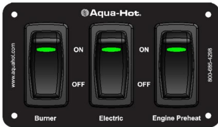
1. Move the Interior Switch Panel's Diesel-Burner switch to the "OFF" position.
