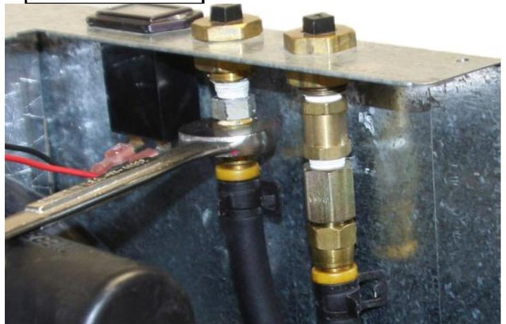
1. Locate where the fuel lines on the diesel burner connect to the Hydro-Hot Bulkhead fittings.
