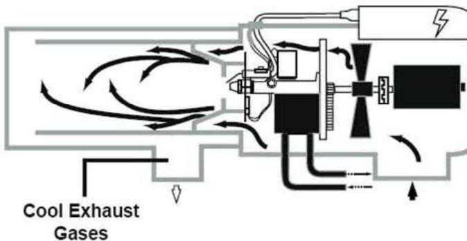
**NOTE:** Whenever the Diesel Burner is switched OFF by the Control Thermostat/ETS Module, it will automatically be reactivated once the Aqua-Hot boiler tank's coolant reaches the present temperature of approximately 160° F (±5°).
