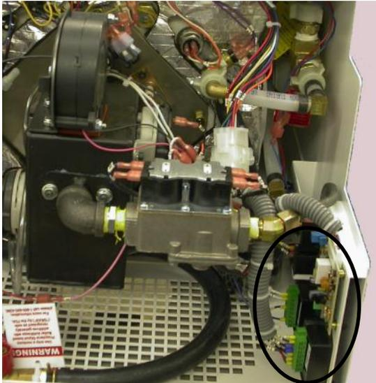
1. Locate both the Propane-Burner's white, electrical plug connection to the Propane-Burner Controller and both of the green plug connections to the Buck Boosts.
