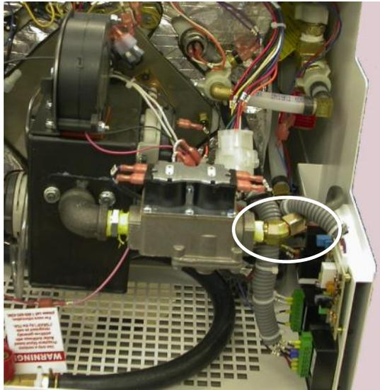
1. Connect the Supply Fuel Line to the Propane-Burner's Gas Valve Assembly.
