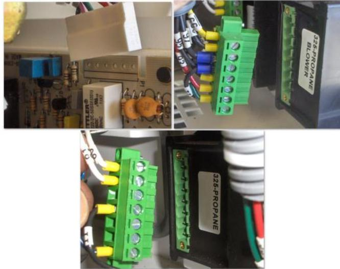
3. Pull the plugs completely out of the Propane-Burner Controller and the Buck Boosts.
