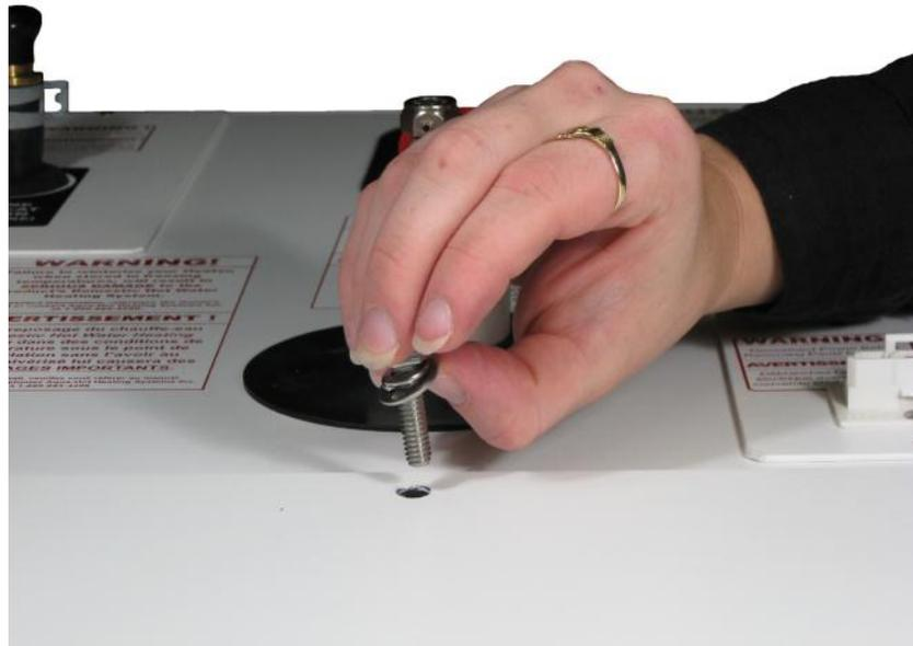
2. Insert the bolts in the two locations on the Aqua-Hot to secure the cover in place; tighten the bolts securely.
