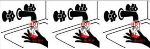
**Risk of Severe Burn or Death from Scalds.** Water temperature over 51°C (123.8°F) can cause severe burns instantly or death from scalds. See instruction manual before setting temperature at water heater. Feel water before bathing or showering. Temperature limiting valves are available, see manual.
