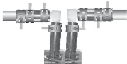
90° Connection Components Installed
